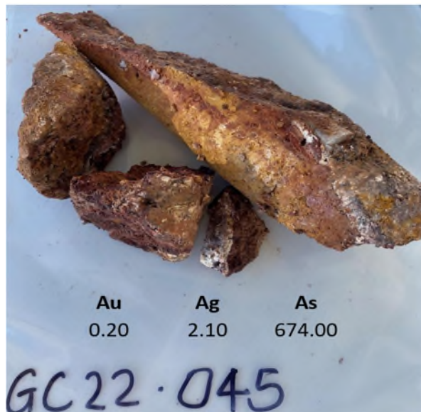
Figure 1. Sample from geochemistry with strong epithermal alteration and quartz veining (all results ppm)
