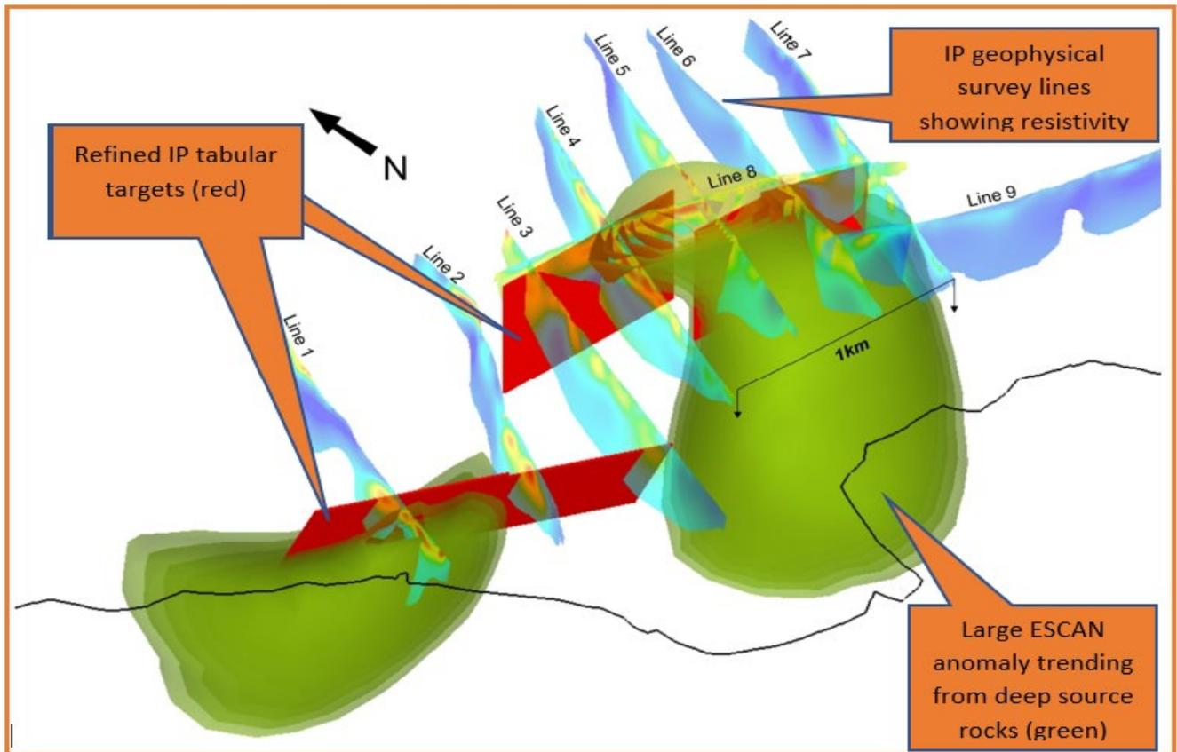
Figure 9 3D image showing ESCAN and IP survey lines with potential gold feeder target zones
