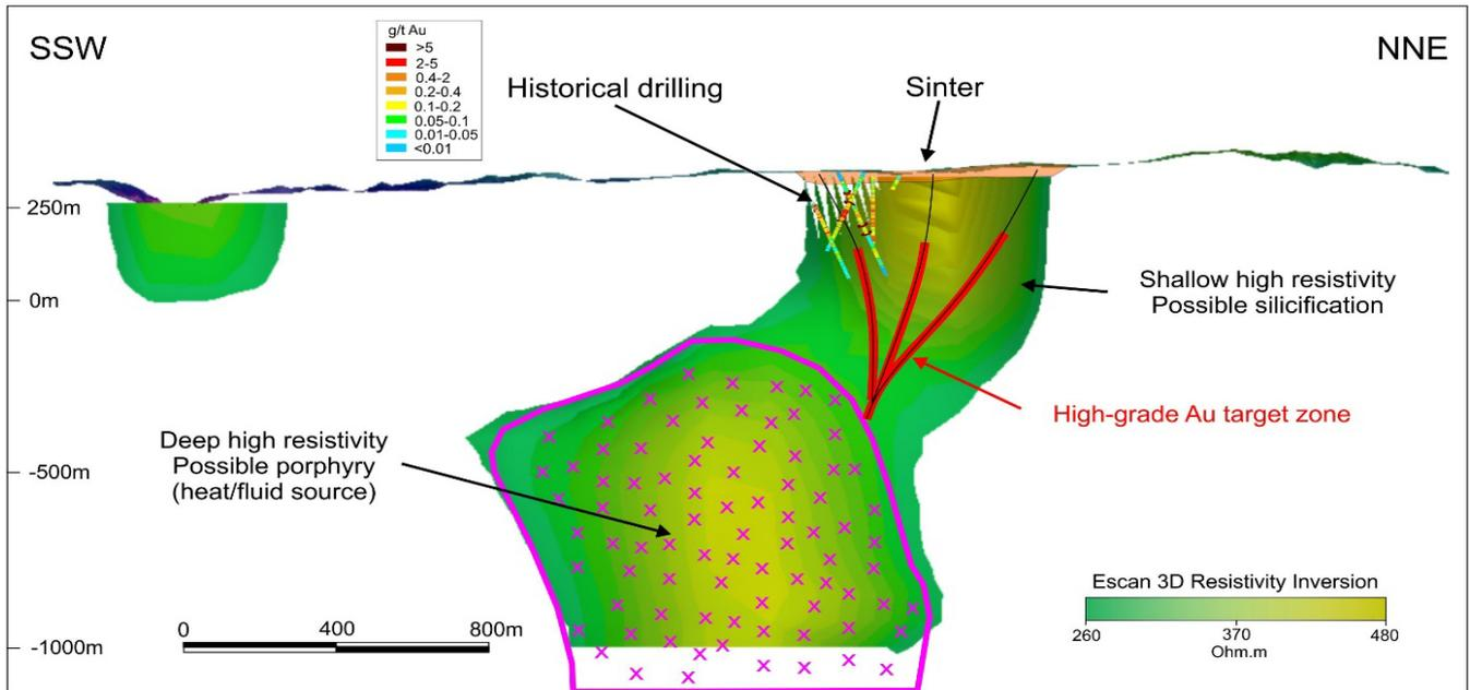
Figure 89 Historic ESCAN anomaly showing deep source and offset from previous drilling
