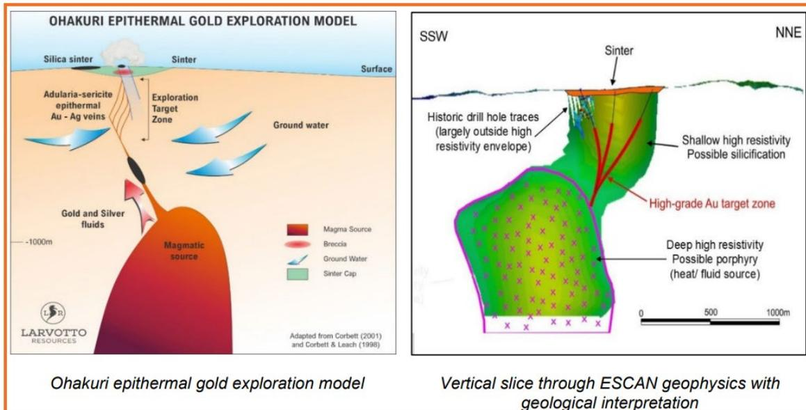
Figure 1213 Ohakuri exploration model (left) and a vertical section of ESCAN showing deep source rocks, feeder zones and historical drilling
