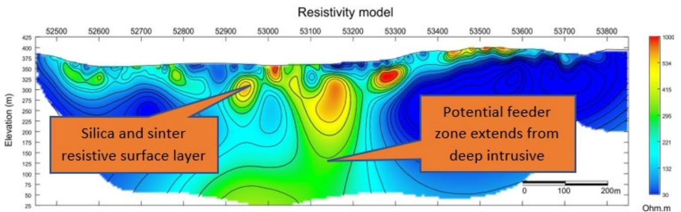
Figure 78 Survey line 8 (along strike) showing resistive potential feeder zone extending to depth
