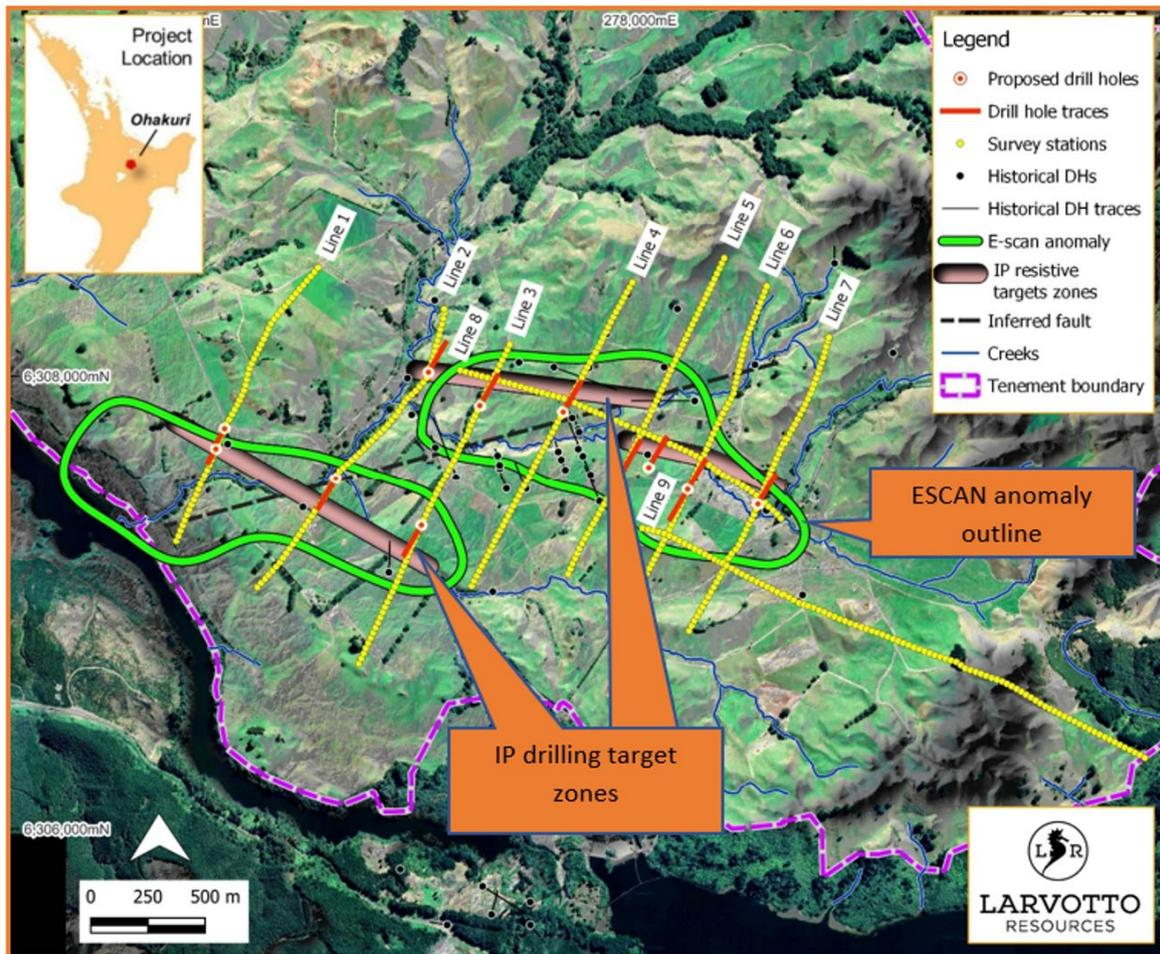
Figure 5.6 Location diagram showing new survey lines and outline of historic broad ESCAN, historic drilling and proposed new drill holes
