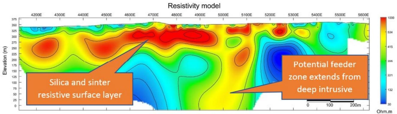
Figure 67 Survey line 6 (across strike) showing potential feeder zone extending to surface from a deep intrusive source
