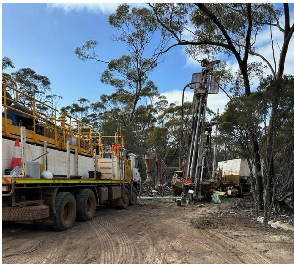
*Figure 4 RC Drilling at Merivale Prospect*
