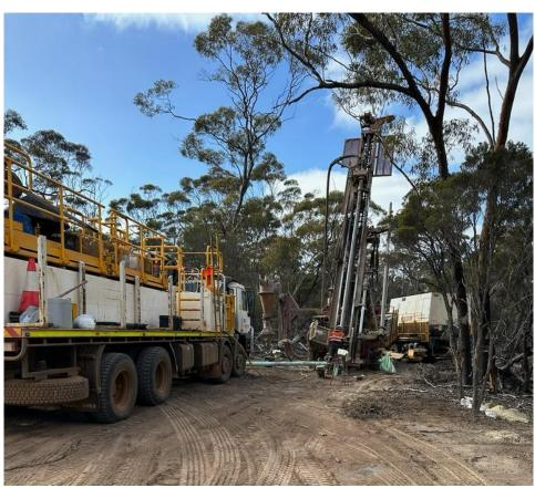
Figure 4 RC Drilling at Merivale Prospect
