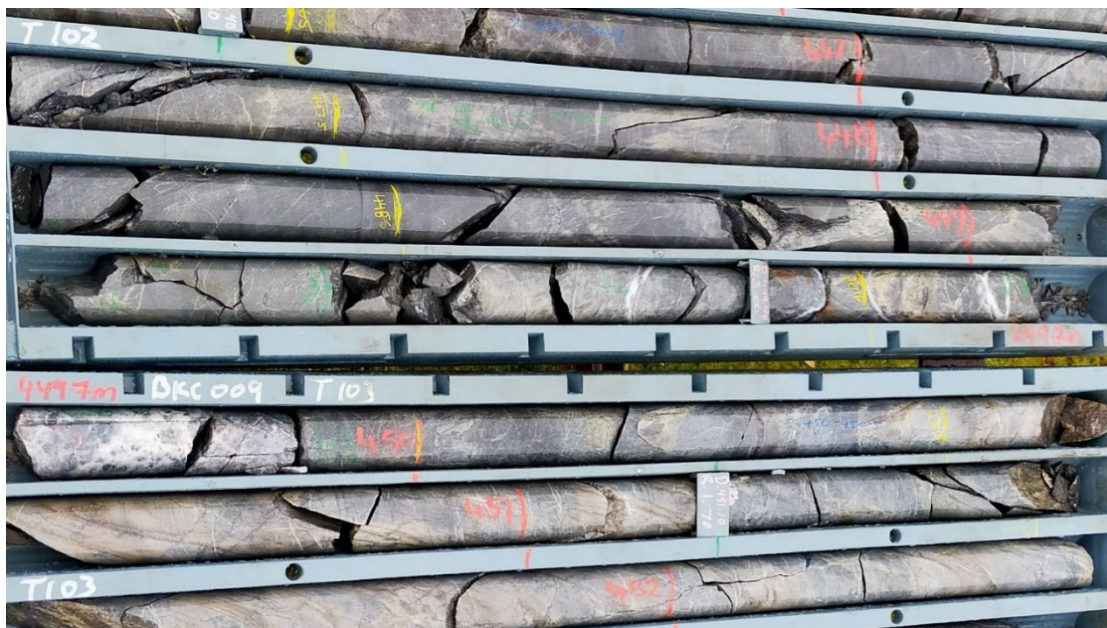
Figure 8 Core tray BKC009 displaying breccia between 449.6 and 450m containing 96.8 g/t Au
