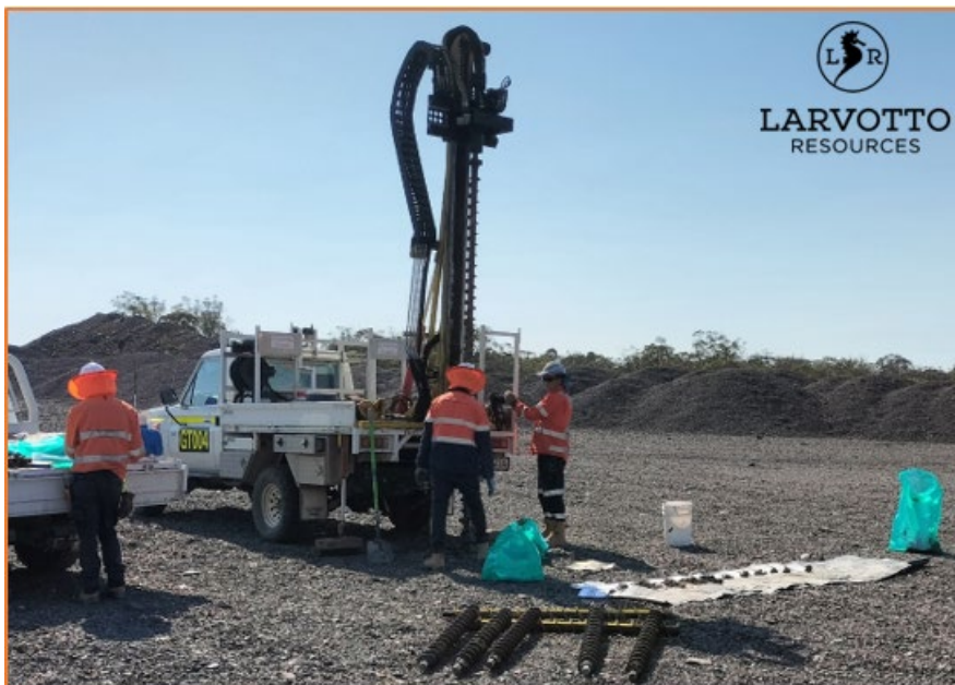
Figure 6 Auger Drilling on the Hillgrove Mines Historic TSF1
