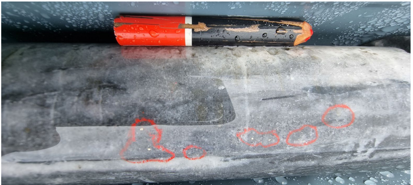
Figure 6 Visible gold identified in core (red circles) in BKC015 from between 245.3m - 250.3m with stibnite, all within quartz-carbonate breccia hosted in highly siliceous meta-siltstone
