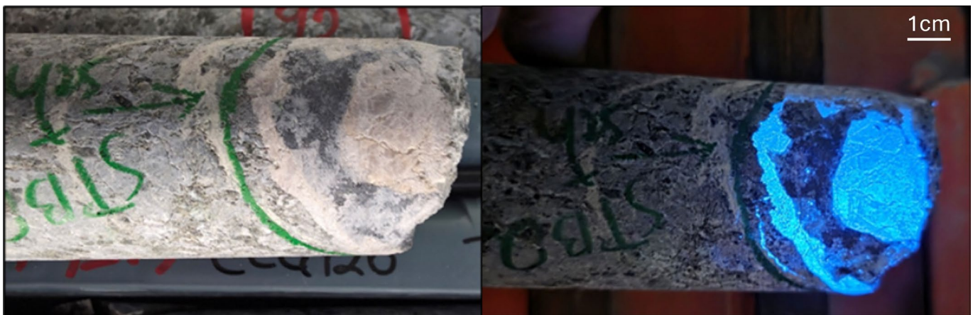
Figure 6: Scheelite (tungsten) mineralisation in CLG126 diamond drill core. Fluorescence observed under UV light.
