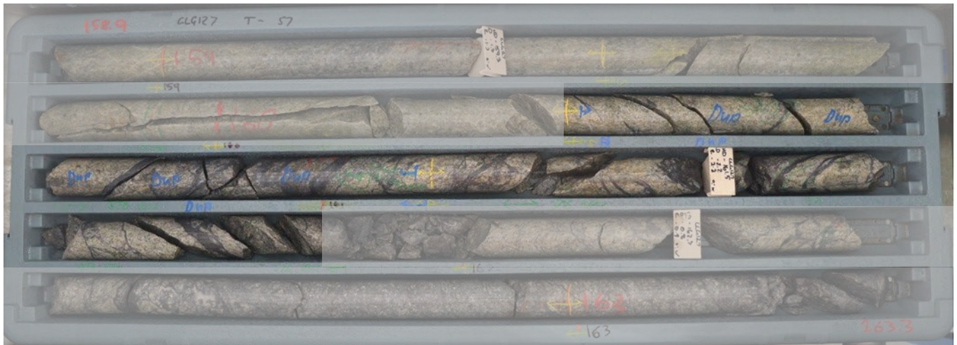
Figure 5: Photograph of CLG127 drill core c. 160.4-162m down hole showing intense stibnite veining (1.60m @ 22.81 g/t AuEq).
