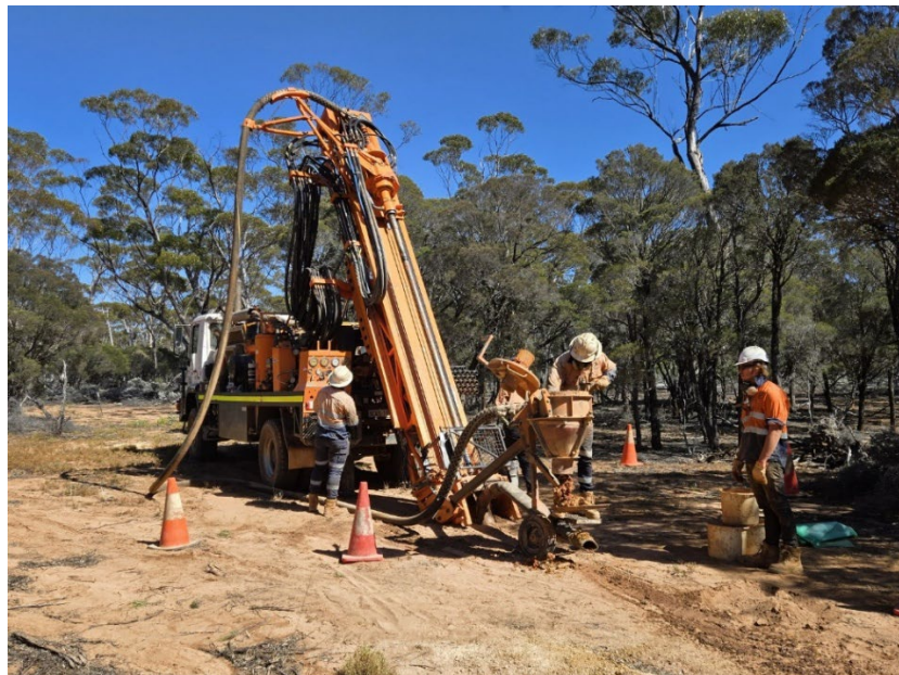
Figure 9 - Aircore drilling at Merrivale South REE prospect
