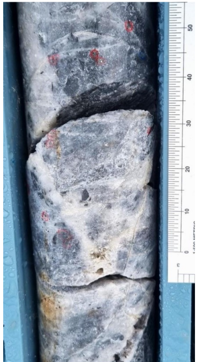
Drill core from BKC018 at 412.6m depth interpreted to be in the Little Reef mineralised zone. Assays for the interval 412.6 to 413.36m returned 104.29 g/t Au and 0.77% Sb. The red-circled points on the core are visible gold grains.
