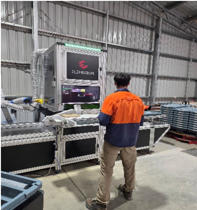
Figure 4 Elemission LIBS Laser Core Scanner in Operation
