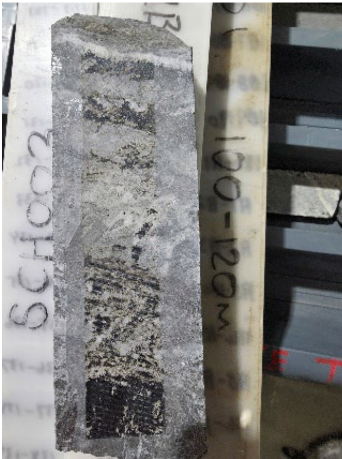
Figure 5 Scanned Core showing area ablated by LIBS laser (darker area) as part of the scanning process
