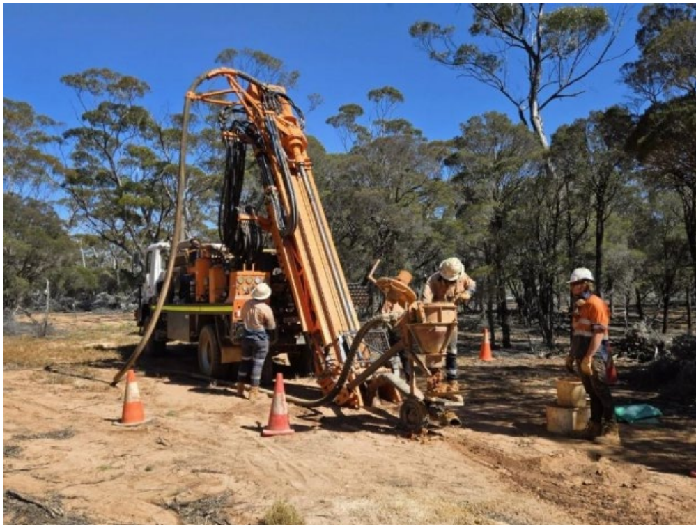
Figure 20 Aircore drilling at Merivale REE prospect
