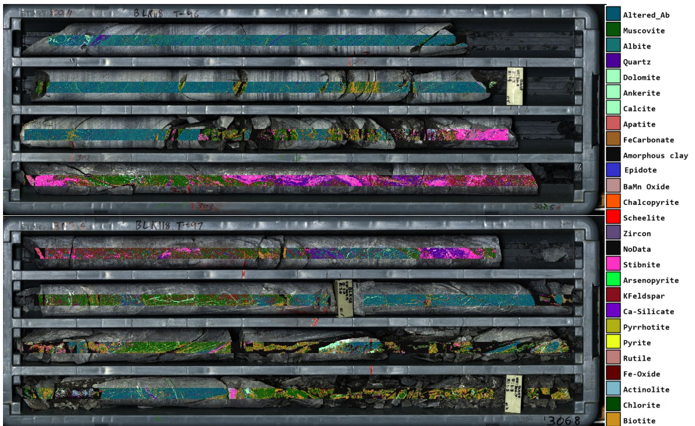
Figure 5 BLK118 LIBS Mineralogy & Core Photos 300.4m - 306.8m (coloured zone) highlighting thick zone of stibnite-quartz mineralisation (pink) and arsenopyrite (green) which hosts gold from 301.8m - 306.8m.
