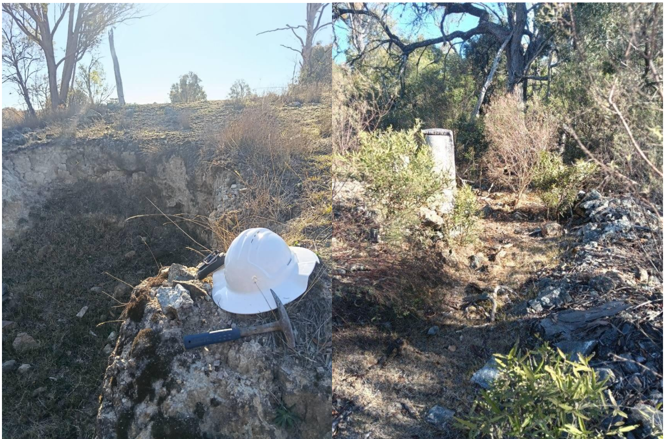
Figure 4 - Historic Workings at Curry's. Left: Shallow artisanal open-pit excavation developed along the Curry's line of workings, reflecting early small-scale mining focused on near-surface mineralisation. Right: Historic prospecting costean excavated along the same line of workings, with mullock and spoil material evident along the eastern (right-hand) margin of the excavation. These workings highlight the extent of historic ground disturbance and provide evidence of continuous mineralised trends at surface.
